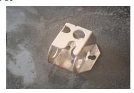
Cut off the tabs at the back of the gearbox. Rub down the back of the gearbox on a flat surface. At this stage the gearbox frame may be blackened. Dry completely before continuing.
