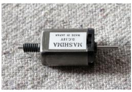
Gently press the worm home on the shaft; you need the motor to turn smoothly but with minimal float on the shaft at this stage.
