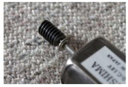
Assemble the washer and worm on to the motor front shaft.
