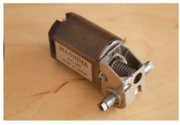
At this stage I lubricate the gears with a little gear lubricant.
