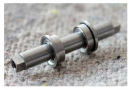
Test fit the bearings on to the axle. If it's too tight then, polish the axle with emery paper until the axle just fits. Do not fix at this stage.
