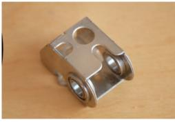
Fix the two bearings with retaining compound. Loctite 603 is recommended.
