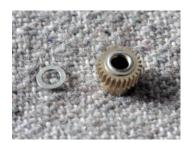
**Note:** The larger washers always fit with the gear in this position. The shaped sides of the washers should always be away from the gear.
