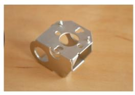
Bend down the second top ear to  $90^{\circ}$ . Twist the tabs on the backplate to lock the two ends together. Solder round all the folds and joints.
