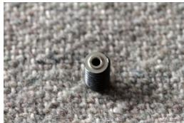
**Note:** The small washer always fits with the worm in this position. The shaped side should always be away from the worm.
