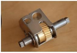
Fit the axle, gear and washers into the gearbox. At this stage test that the axle turns over smoothly.
