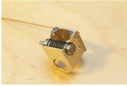
Test fit the worm shaft and bearings in to the gearbox frame.
