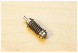
Assemble the washers, bearings and worm on to the silver steel shaft.
