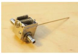
Replace the worm unit, bearing holders and screws and adjust the mesh of the gears by sliding the holders up and down in the frame, before locking off the screws.
