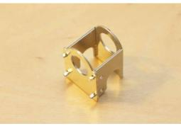
Twist the tabs to lock the parts together.
