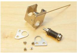
Removing the screws will allow this entire assembly to be separated from the gearbox and also provides a means of adjusting the mesh of the gears when finally assembled.
