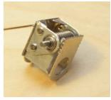
Fit the bearing holders to the frame, both front and rear.
