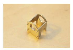
Check that the sideplate and the main part of the gearbox fit together easily on the tabs. If you find that any of the tabs are too tight they can be eased now. Do not solder at this stage.
