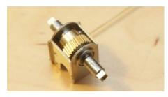
Test fit the axle, gears and washers into the gearbox. At this stage test that the axle turns over smoothly.
