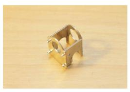
Tap the holes in the frame M2 for the provided screws.
