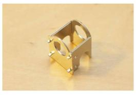
Run solder around the joints and folds.
