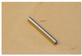
Cut the shaft to a suitable size for your application. De-burr both ends  $% \left( 1\right) =\left( 1\right) \left( 1\right) \left$
