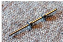
Test fit the bearings on the 2mm diameter silver steel shaft. If it's too tight then you can polish the motor shaft with emery paper until it just fits. Do not fix at this stage.
