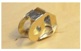
The joints and all other bend lines can now have solder run in. Take care to ensure that solder does not get on to the surfaces that seat the bearings.
