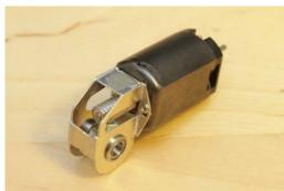
Fit the motor and worm to the gearbox.
