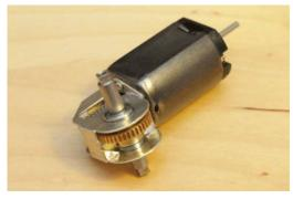
Test fit the axle, gear and washers into the gearbox.
