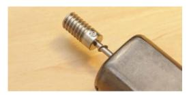
Assemble the small washer and worm on to the motor front shaft.
