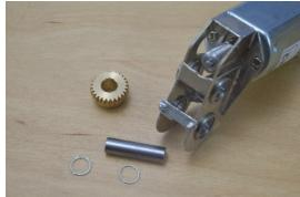
Fit the 26 tooth gear, washer and stub axle into the gearbox
