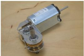
Test fit the axle, 40 tooth gear and washers into the gearbox.
