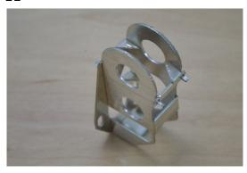
Bend the triangular ear on the strap, fit to the gearbox with the ear on the same side as the others. Twist the tabs protruding through the strap.
