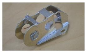
The joints and all other bend lines can now have solder run in. Take care to ensure that solder does not get on to the surfaces that seat the bearings.
