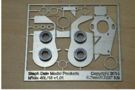
The bearing holes have been reamed for you. Test fit the bearings in the holes as shown. Do not fix at this stage.
