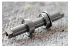
Test fit the bearings on to the axle. If it's too tight then polish the axle with emery paper until the axle just fits. Do not fix at this stage.
