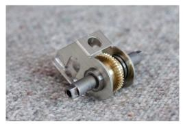
Test fit the axle, gear, washers and bearings into the gearbox. Note: These bearings fit with the flanges on the inside of the gearbox.
