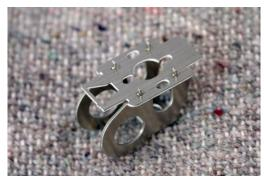
Check that the sideplate and the main part of the gearbox fit together easily. Test the tabs and slots carefully, one set at a time. If you find that any of the tabs are too tight they can be eased now.
