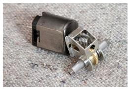
Thread the worm gear on the motor shaft as the gearbox is mated with the front of the motor.
