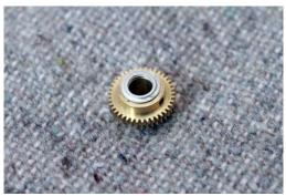
Note: The washers always fit with the gear in this position. The shaped sides of the washers should always be away from the gear.
