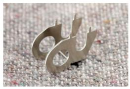
BBend up the two sides, each to  $90^{\circ}$ . The half-etched lines are on the inside of the fold.
