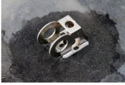
Rub down the back of the gearbox on a flat surface.
