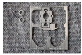
Remove the two shaped washers from the fret.
